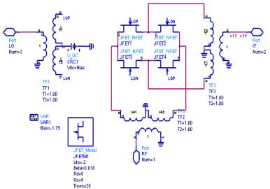
$$I_{DS} = \beta V_{DS} [2(V_{GS} - V_T) - V_{DS}] (1 + \lambda V_{DS})$$
