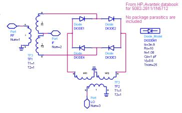
and D1) on. This switching action causes mixing of the RF signal applied to the diodes by the other transformer. This is a broadband mixer, limited mostly by the physical construction of the transformers. Typical commercial mixers such as the MiniCircuits JMS-1 will operate for LO and RF signals from 2 to 500 MHz.
