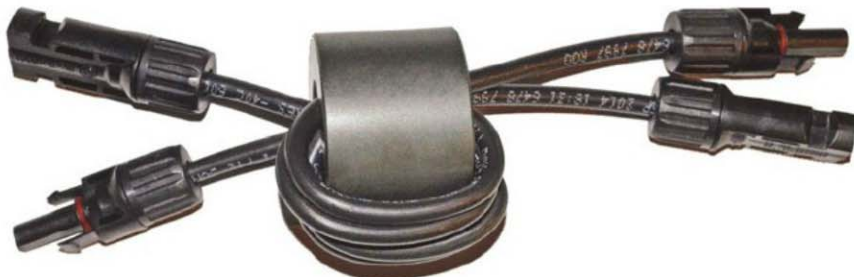
Figure 5 — Three bifilar turns of #10 PV wire on Fair-Rite 2631626202 core with MC4 connectors installed.
