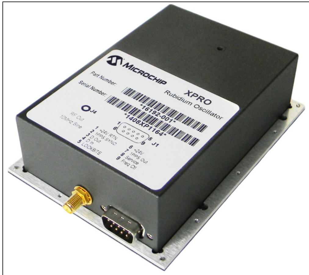
FIGURE 1-1: XPRO High-Performance Rubidium Oscillator.
