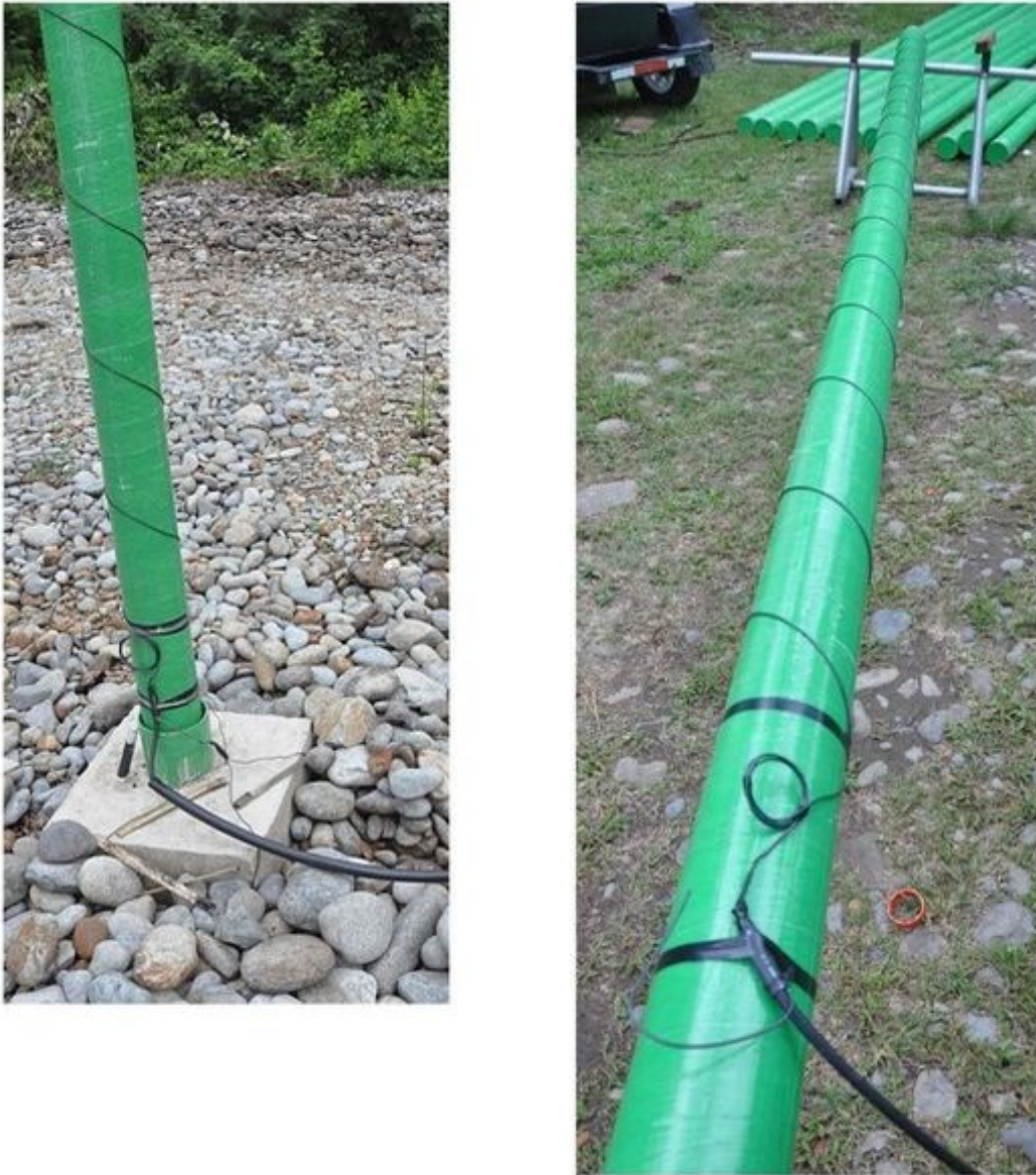
Figure 6. Normal-mode helical monopole with air-coil on a fiberglass mast (8 MHz).
