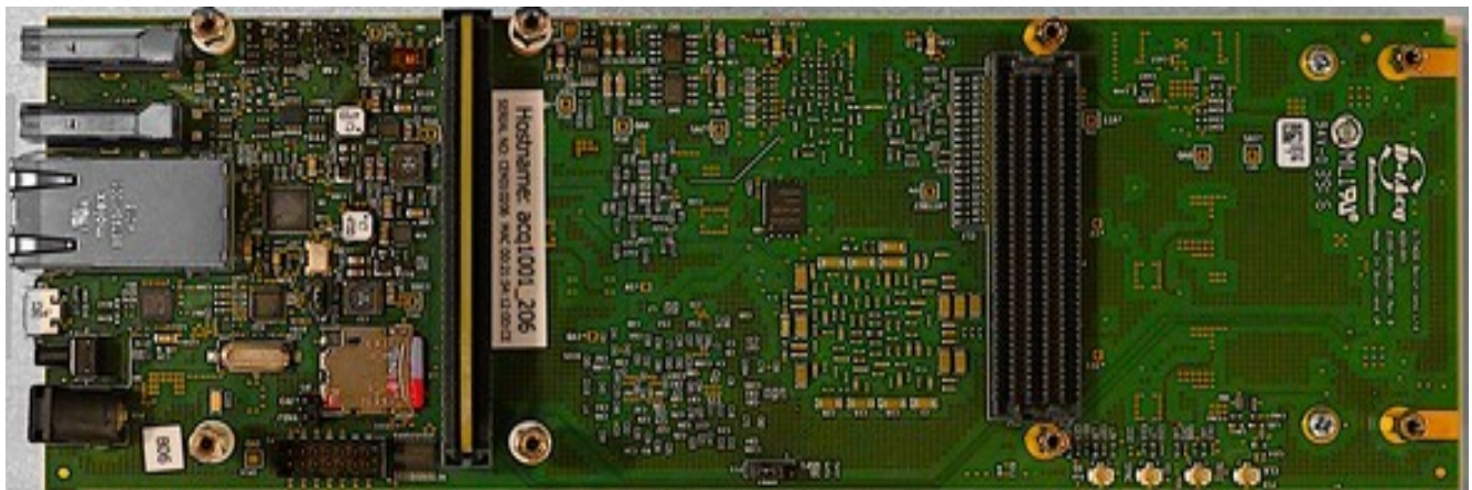
Figure 3c. Photo of the carrier board with FPGA (top face; bottom face not accessible).
