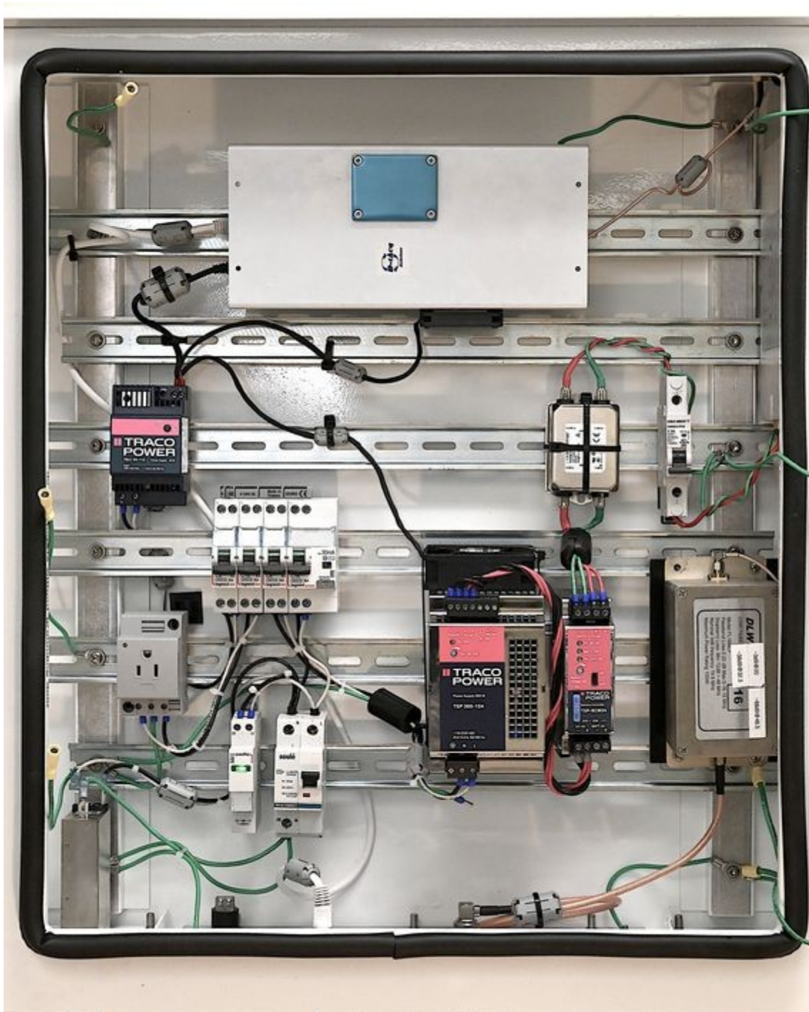
Figure 9. Synthesizer-Transmitter Unit, door open. Bottom rails: power supplies with circuit breakers. Upper rail: digital synthesizer and controller with blue thermal bell. On the right wall: the power amplifier module and the low-pass filter.
