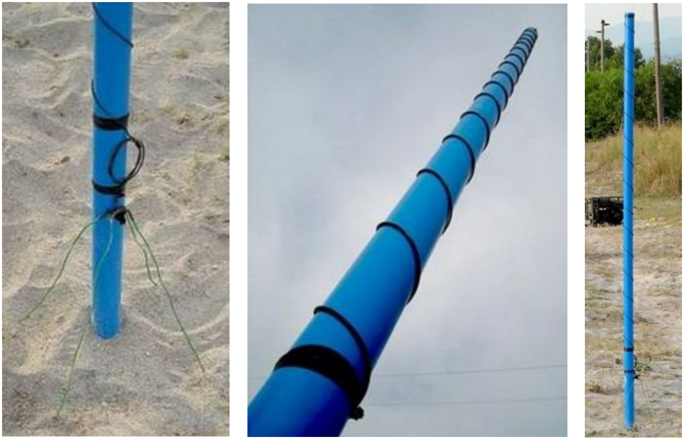
Figure 7. Normal-mode helical monopole with air-coil on a PVC mast (16 MHz).
