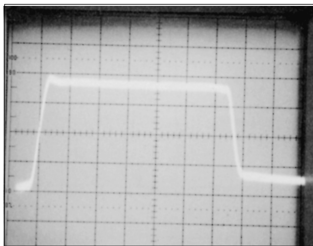
Fig 41—TDR display of the impedance characteristics of the 142-foot Hardline run to the 432-MHz antenna at KD5HM. The scope is set for 0.05 ms per division. See text for discussion.
