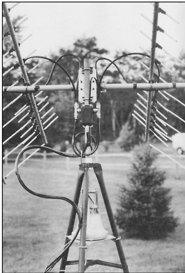
Fig 47—Rotator loop for UHF Yagi array. The feed coax is bundled with a control cable for the polarization relay. The coax/control-cable loop is taped to the rotating mast and to the top of the tower with vinyl electric tape to allow the array to be rotated.
