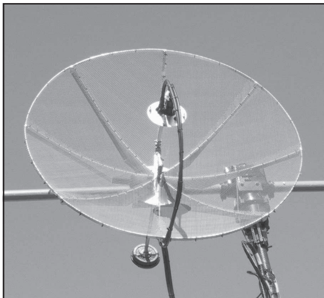
Fig 37—Prototype 1.2-meter dish by Rick Fletcher, KG6IAL, using a dual-band (L and S) patch-feed antenna for AO-40. See text. This kit dish is covered with 1/4-inch mesh. (KG6IAL photo.)
