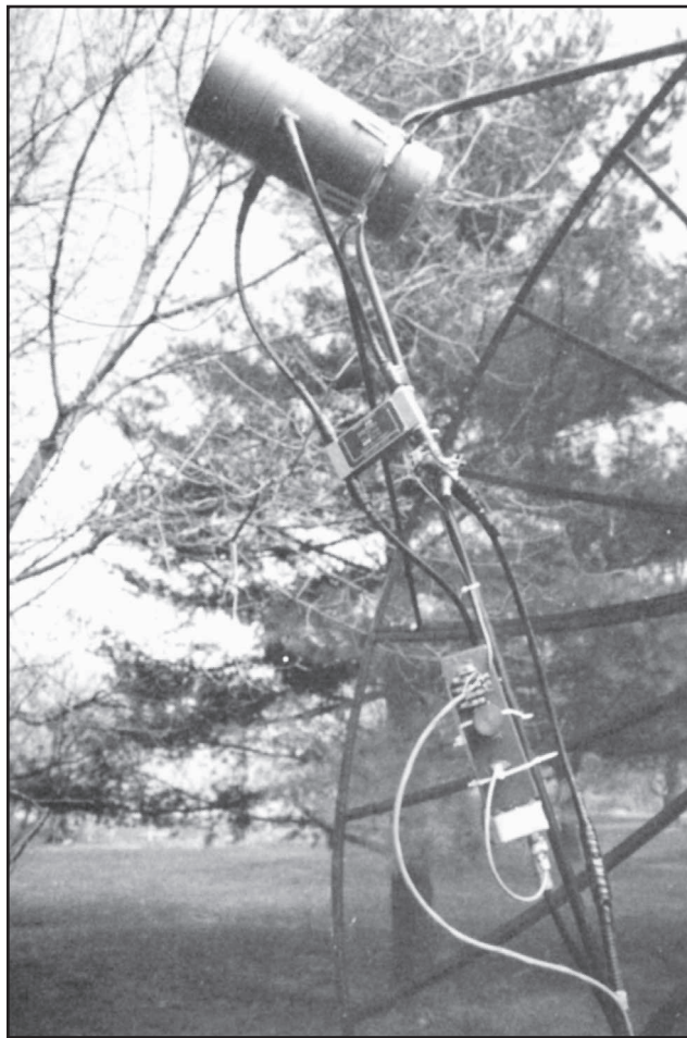
Fig 92—View of feed, showing coffee-can feed horn and hybrid coupler.
