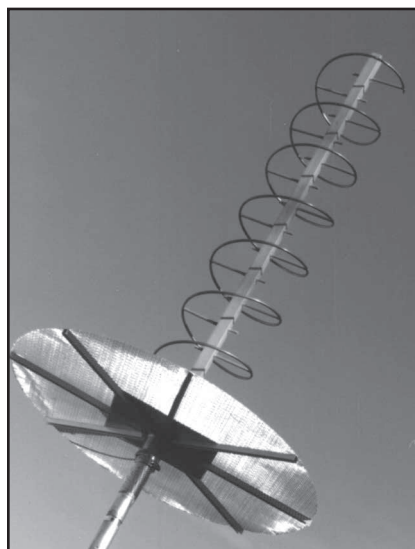
Fig 56—The portable 435-MHz helix assembled and ready for operation. (WØCY photo.)
