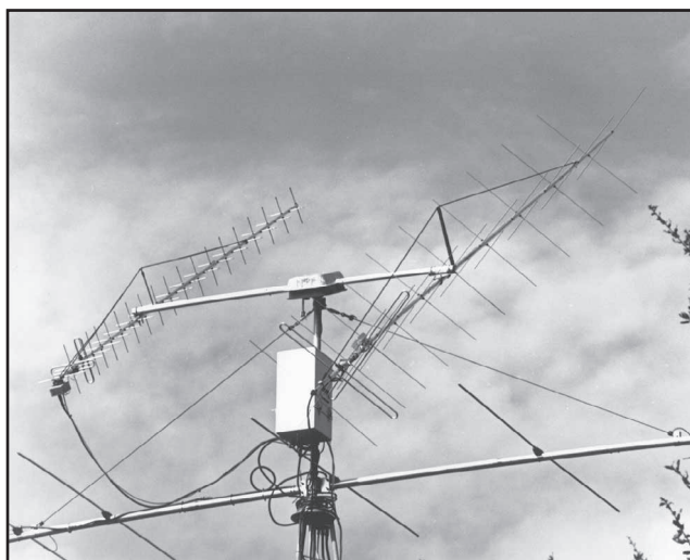
Fig 6—Dick Jansson, WD4FAB, used these 2-meter and 70-cm crossed Yagi's in RHCP for AO-10 and AO-13 operations. The satellite antennas are shown mounted above a 6-meter long-boom Yagi.
