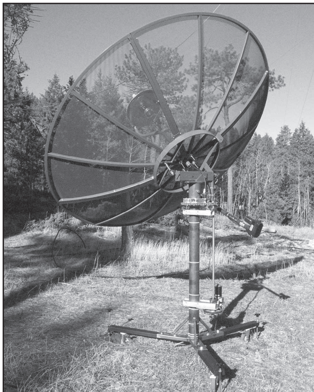
Fig 69—A completed TVRO dish Az-EI mounting system is shown, using a jackscrew elevation drive. (W0LMD photo.)
