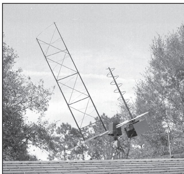
Fig 15—At top, a seven-turn LHCP helical antenna for S-band dish feed for AO-40 service. This helical antenna uses a cupped reflector and has a preamplifier mounted directly to the antenna feed point. At bottom, a pair of helical antennas for AO-10 service on 2 meters and 70 cm. The 2-meter helical antenna is not small! (WD4FAB photos.)
