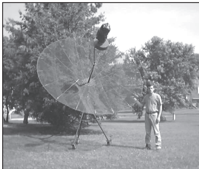
Fig 87—N2UO's homemade 12-foot stressed dish. (Photo courtesy N2UO.)
