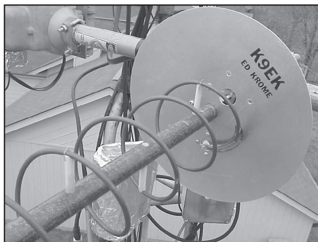
Fig 59 —At top, the method of reinforcing the reflector screen with aluminum channel stock is shown. In this version of the antenna, the three angle brackets of Fig 58 have been replaced with a surplus aluminum flange assembly. ( W0CY photo. ) At bottom, this helix view shows the details of a \frac{1}{4} -turn matching transformer, as discussed in the text. ( K9EK photo. )
