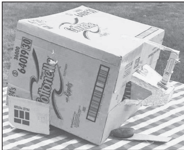
Fig 35 —Side view of the downlink pyramidal horn showing the elevation control supports and how the downconverter is attached to the horn. The downconverter is pulled forward by the tape to align the probe wire parallel to the rear surface of the horn.
