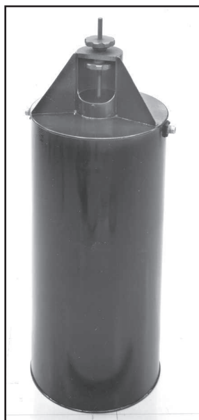
Fig 16—A coaxial cavity filter of the type used in many amateur and commercial repeater installations. Center-conductor length (and thus resonant frequency) is varied by adjustment of the knob (top).
