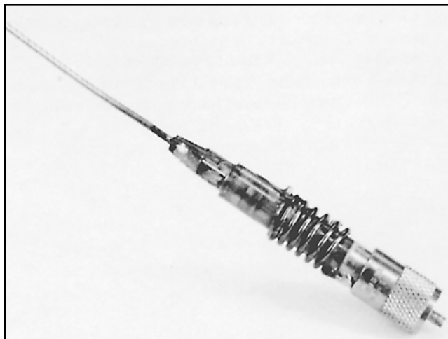
Fig 51—The 220-MHz \frac{5}{8} - \lambda mobile antenna. The coil turns are spaced over a distance of 1 inch, and the bottom end of the coil is soldered to the coax connector.
