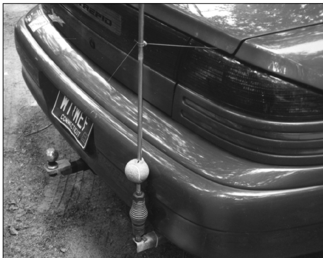
Fig 2—A typical bumper-mounted HF mobile antenna, as used by W1WEF. Note the nylon guy lines and the tennis ball used as a shock absorber. (Photo courtesy W1WEF.)
