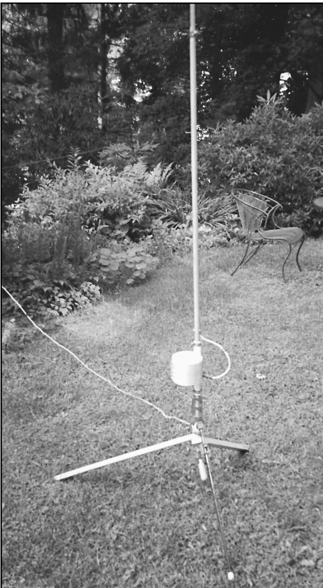
Fig 6 —At top, the portable antenna in some of the many places it may be mounted around the house, porch and yard. At bottom, the simple ground-mounted legs that make a tripod.
