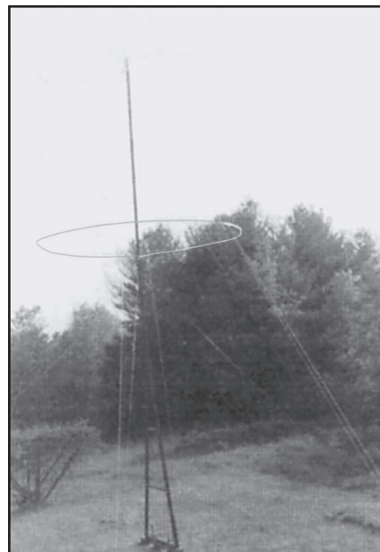
Fig 52—Photo of W8NWF's original A-frame mounted HF discone.
