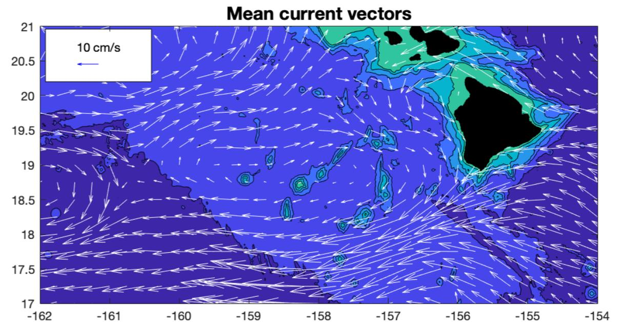
The bathymetry of South Point and associated mean currents.
