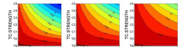
SSTA response (local minimum) from numerical experiments by varying TC strength and wind duration forcing time
