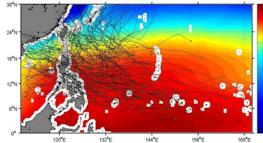
Regional map showing the tracks of tropical cyclones during the period 2003-2012, with green circles indicating where they are formed. The background color is the satellite-derived mean SST ( $^{\circ}\text{C}$ ) from 2003 to 2012.
