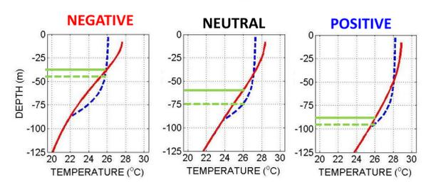
SST profile before and after passage of Category 3 typhoon with a moderate Translation Speed (Wind Forcing = 3 hours) at different background profiles (red line are pre typhoon profile; blue broken line are post typhoon profiles; green lines are the location of D26)
