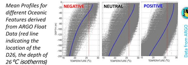
Mean Profiles for different Oceanic Features derived from ARGO Float Data (red line indicating the location of the D26, the depth of 26 $^{\circ}\text{C}$  isotherms)
