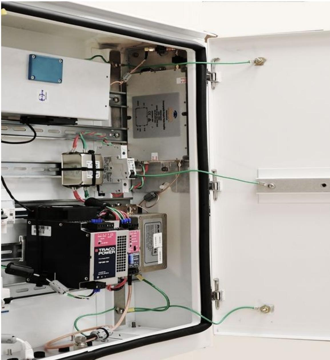
*Figure 2. Synthesizer-Transmitter Unit, door open, slanted view. The power amplifier module (top) and the low-pass filter (bottom) are seen on the right inner wall.*
